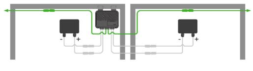
If connecting a TS4-A-2F to only one solar module, connect the TS4 #2 input cables to each other.
